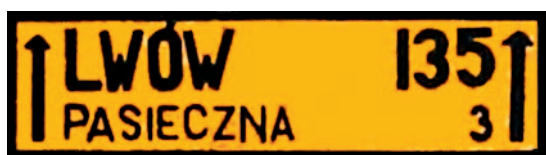
Fig. 1. Direction sign from Polish manual from 1938 (less distant town at the bottom)
